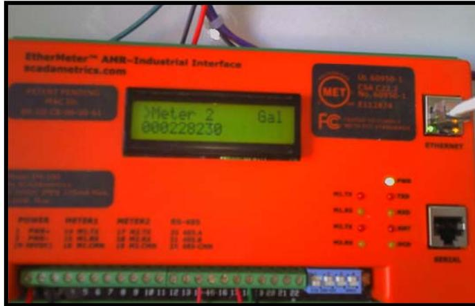
EtherMeter Connected to The 6 Inch MMT Turbo Meter.
