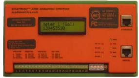
Both EtherNet and Serial (RS-232 and RS-485) communication methods are supported across Allen Bradley's modern control equipment lines. Serial support includes the DF1 Full Duplex and DF1 Radio Modem protocols, and Ethernet support consists of the EtherNet/IPTM protocol.
