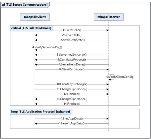
Figure 6 TLS Full Handshake Protocol
