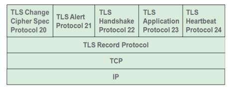
**Figure 2 TLS Communications Protocol Stack**
