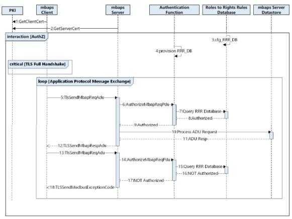
Figure 4 Modbus/TCP Security Concept View
