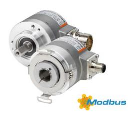
With the new Sendix F5868 and F5888 encoders, Kübler complements its F multiturn family products range with robust high-resolution Modbus encoders with a through hollow shaft up to 15 mm for a compact size of only 58 mm. This through hollow shaft leaves, for example on drives, many possibilities for other motor options located behind the encoder. These gearless optical encoders are based on the innovative and patented Intelligent-Scan-Technology<sup>TM</sup>.
